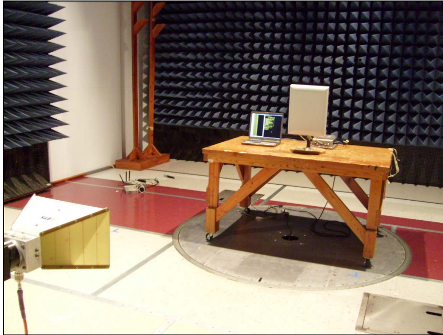
Photograph 8. Test Equipment and Setup for Various Radiated Measurements – 13 dBi Sector
