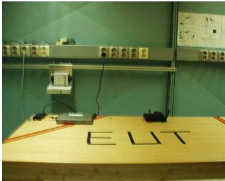
Power line conducted emission
