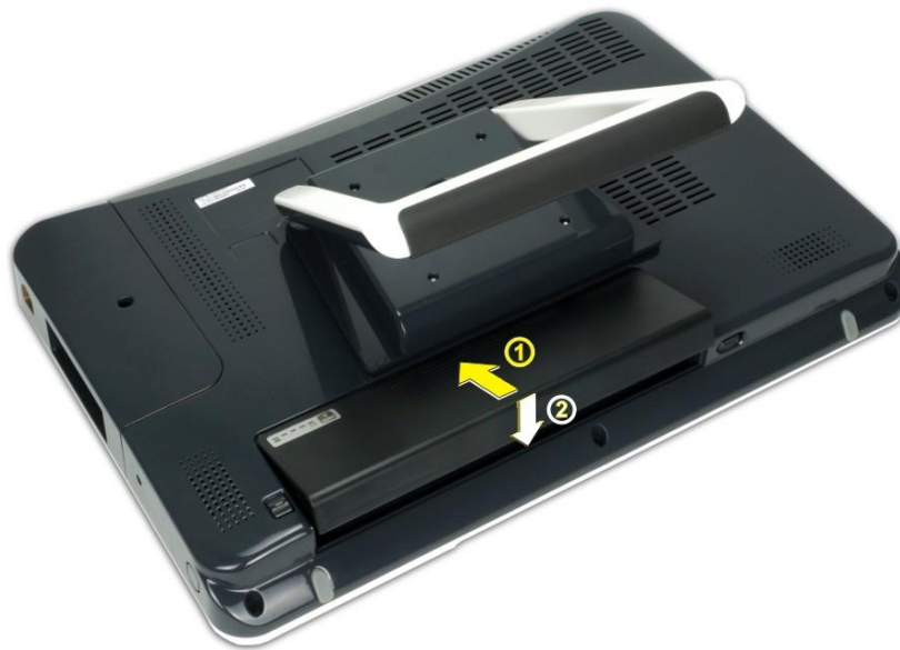
Figure 3-2: Battery Pack Installation
