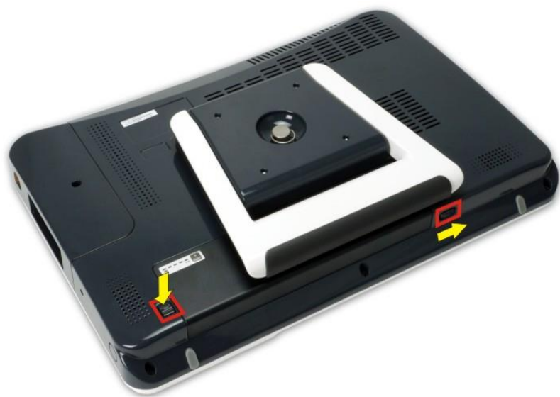
Figure 3-4: Battery Pack Removal
