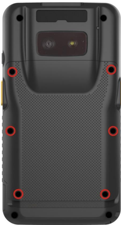
Figure 3-4: Battery Cover Retention Screws
