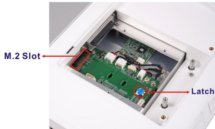
Figure 3-6: M.2 Slot Location
