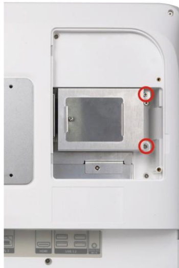
Figure 3-2: HDD Bracket Retention Screws
