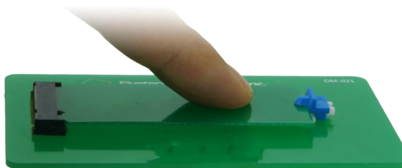
Figure 3-8: Securing the M.2 Module
