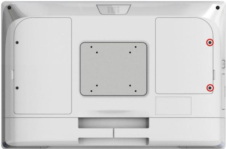
Figure 3-1: HDD Cover Retention Screws
