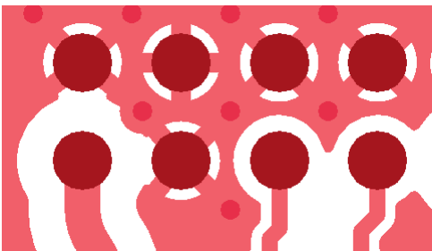
Figure 26: AP antenna port layout recommendation
