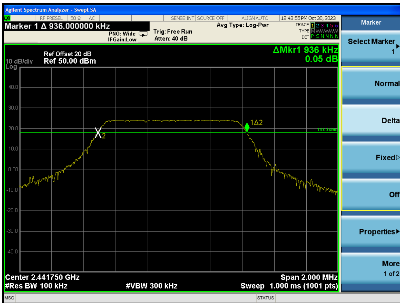
DTS Bandwidth – Middle Channel
