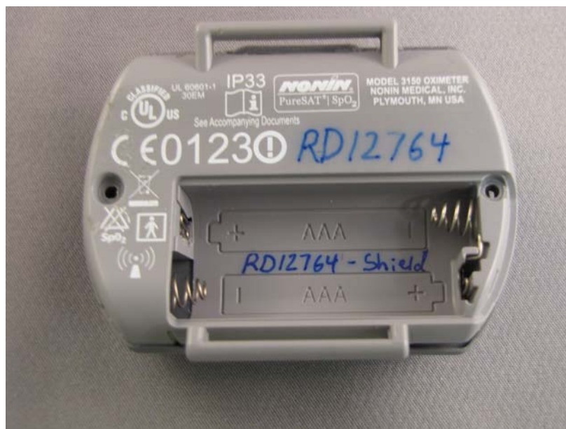
Figure 5 Model 3150 Back showing device label printing
