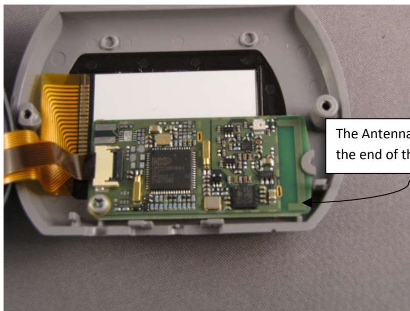
Figure 3 SABER PWBA mounted over LCD in top cover of Model 3150
