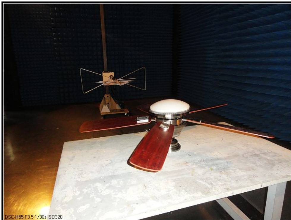
Radiated emission test view--
