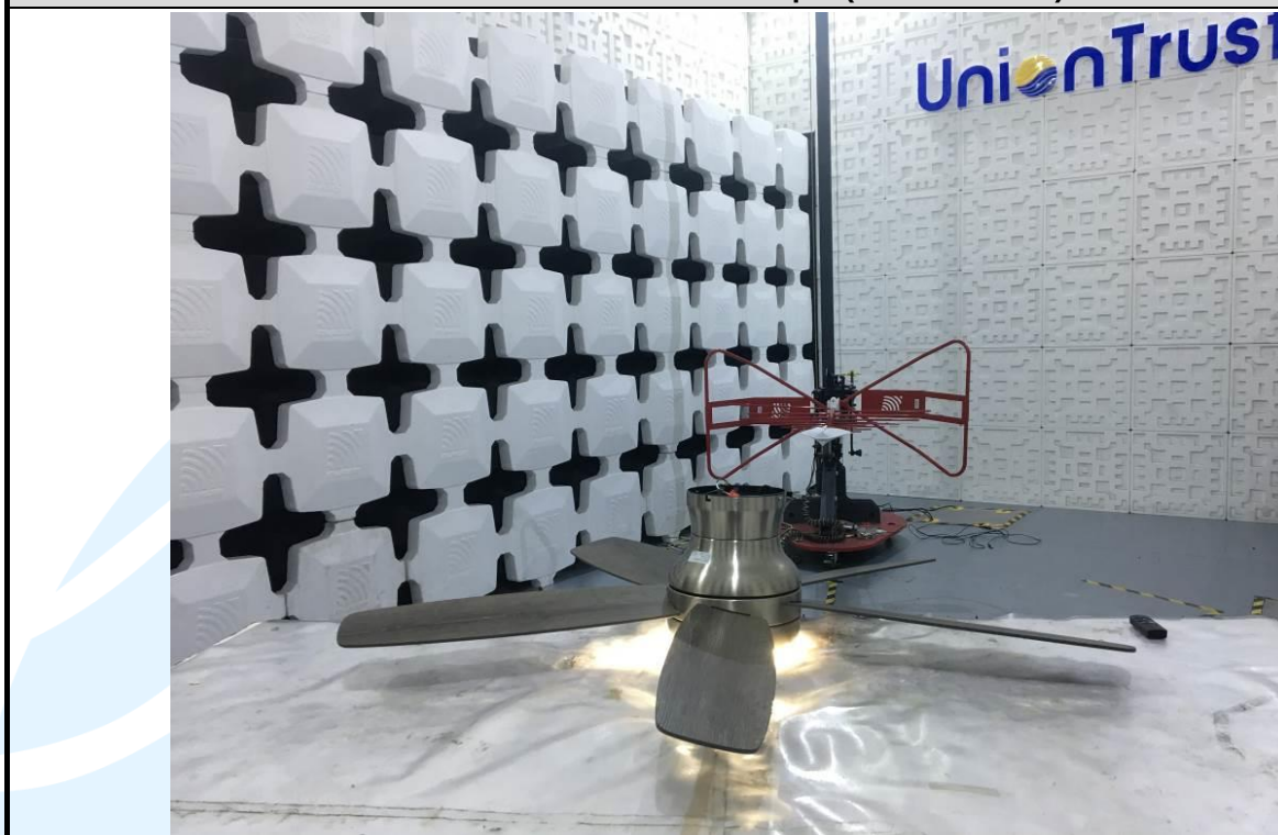
Radiated emission Test Setup-1 (30 MHz~1 GHz)
