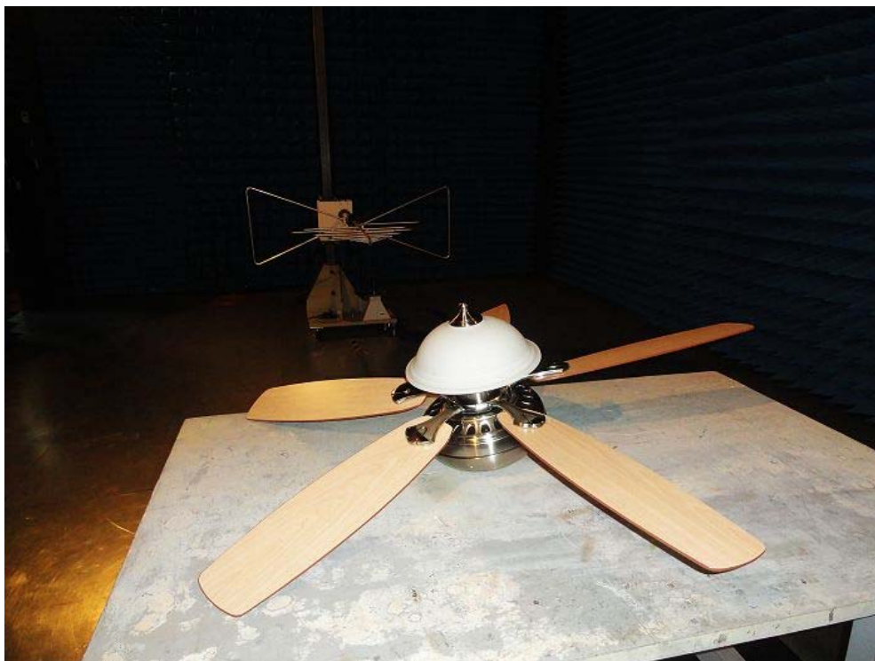
Radiated emission test view--
