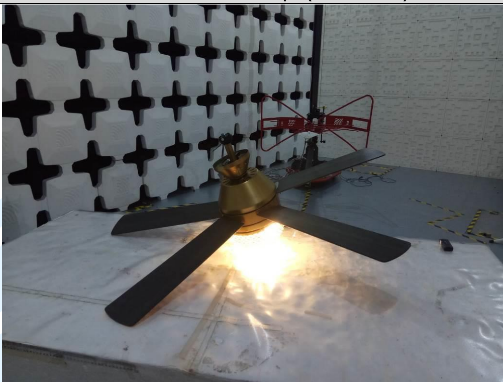
Radiated emission Test Setup-1 (30 MHz~1 GHz)
