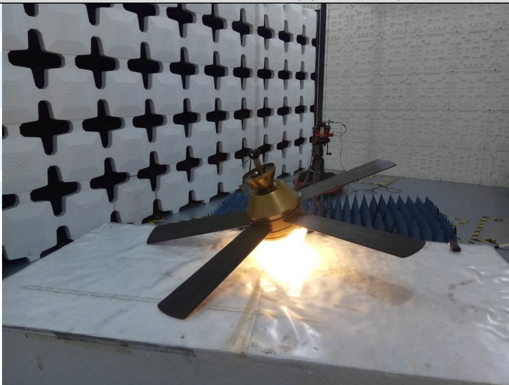
Radiated emission Test Setup (Above 1 GHz)
