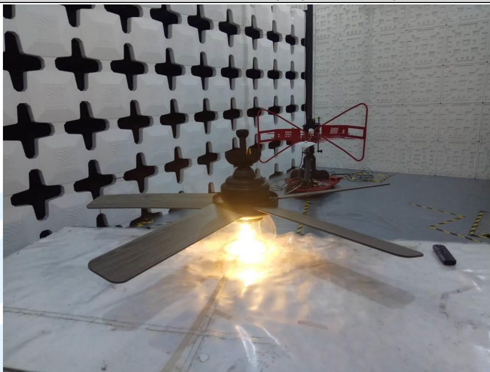
Radiated emission Test Setup-1 (30 MHz~1 GHz)
