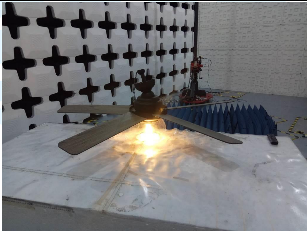
Radiated emission Test Setup (Above 1 GHz)
