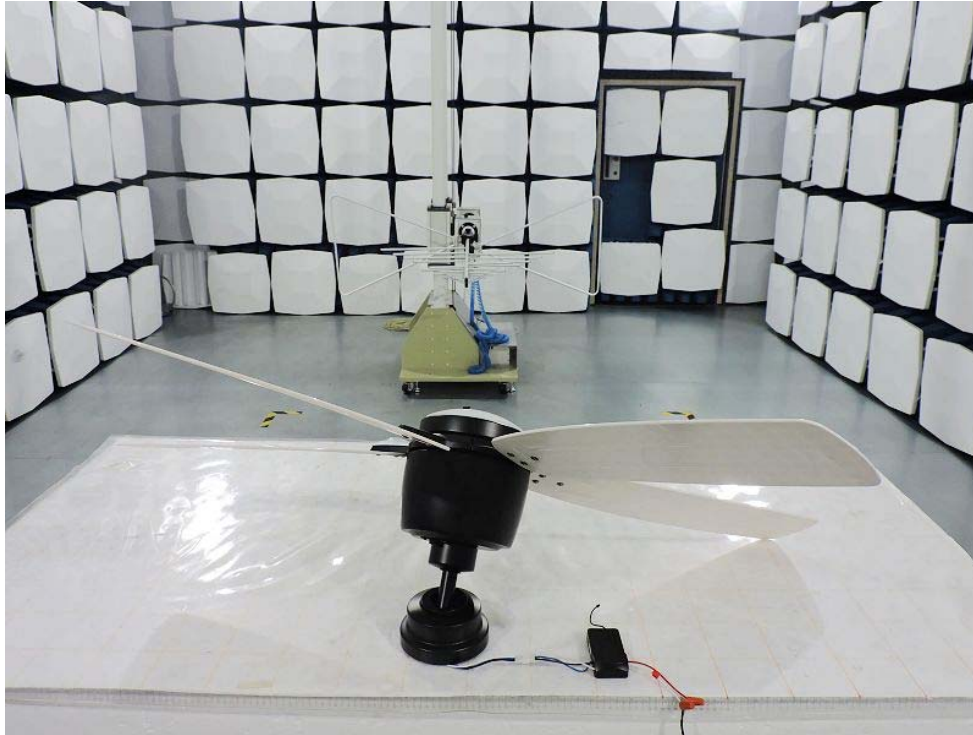
Radiated emission test view—
