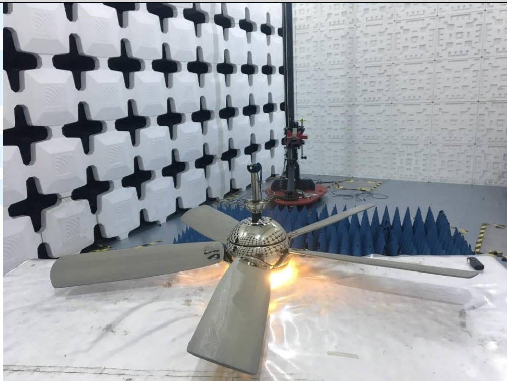
Radiated emission Test Setup (Above 1 GHz)
