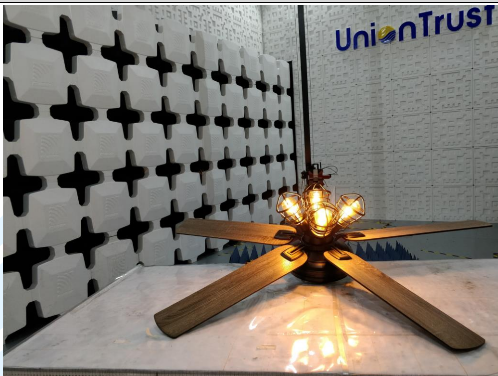
Radiated emission Test Setup-2 (Above 1 GHz)
