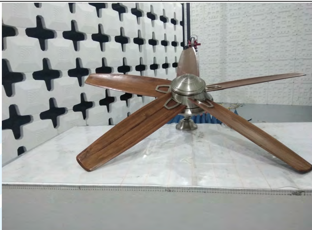
Radiated emission Test Setup-2 (Above 1 GHz) - Mode 1
