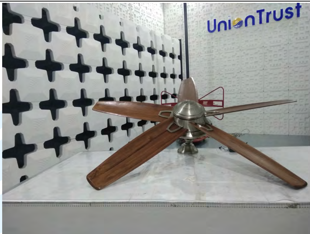
Radiated emission Test Setup-1 (30 MHz~1 GHz) - Mode 1
