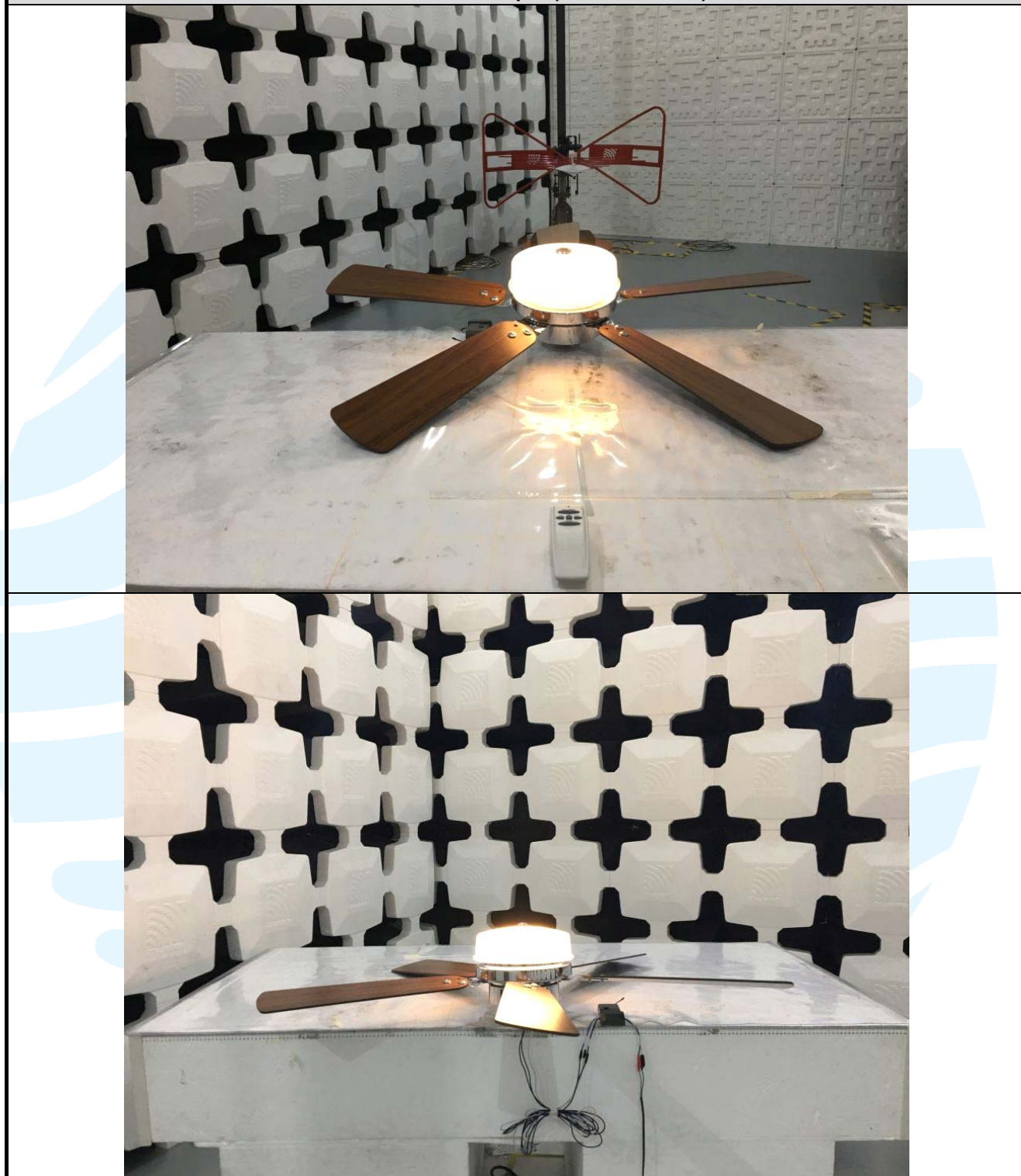
Radiated emission Test Setup-1 (30 MHz~1 GHz) - Mode 1
