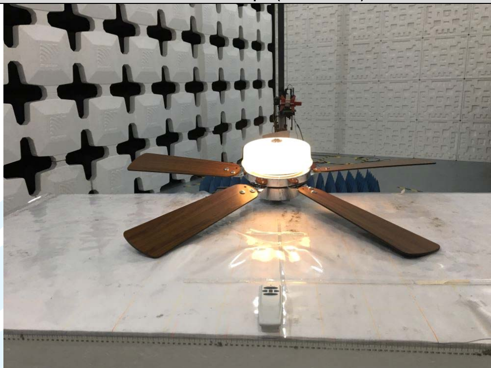
Radiated emission Test Setup-2 (Above 1 GHz) - Mode 1
