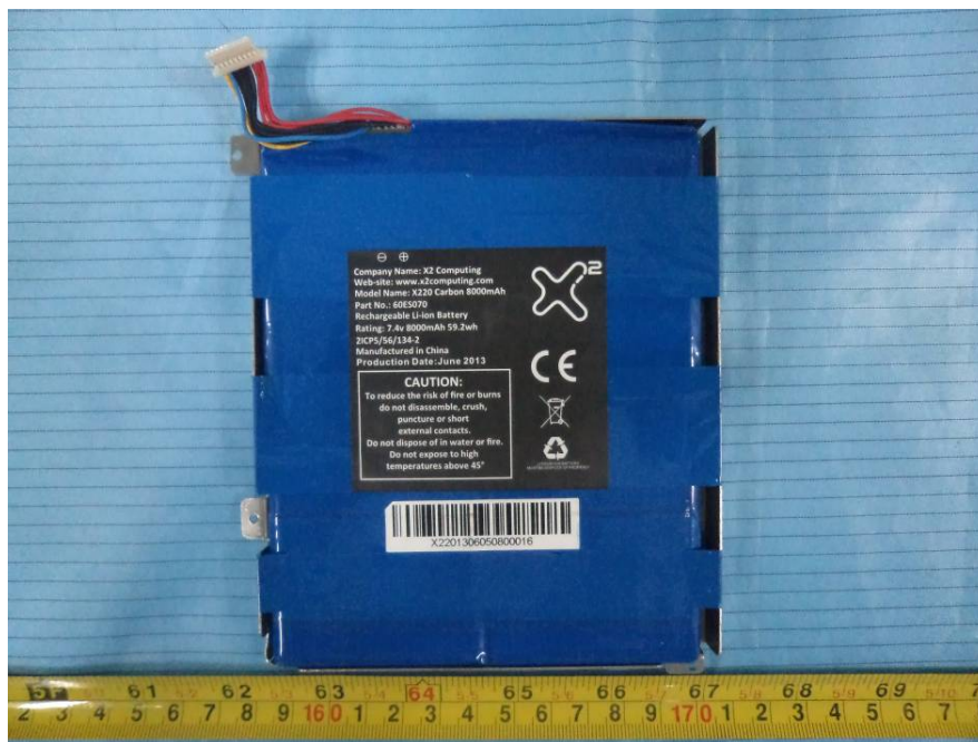
EUT – Battery View (8000mAh)
