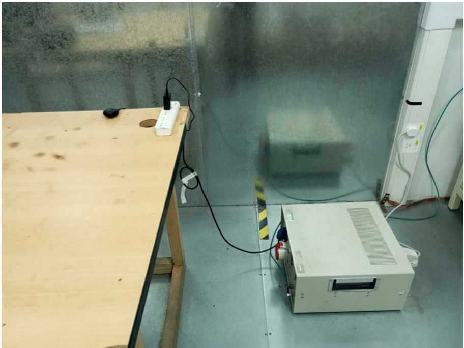
Conducted Emission Test Setup
