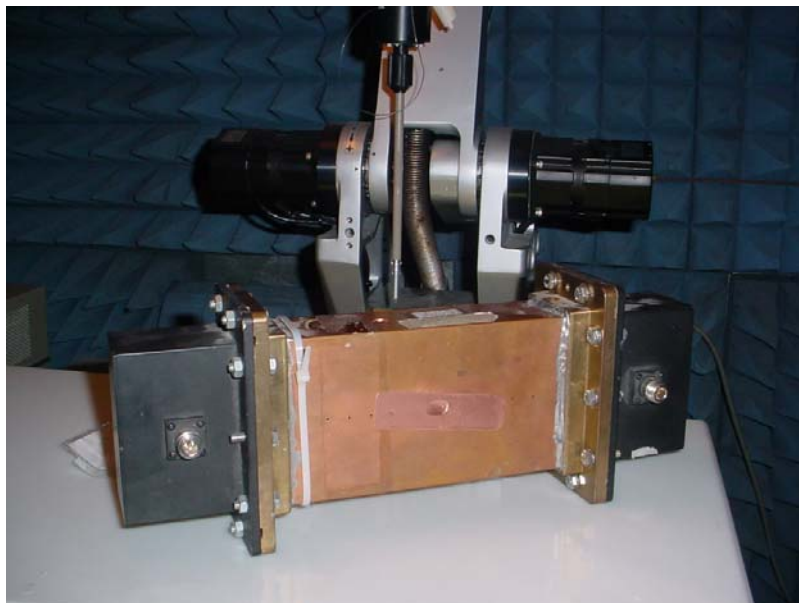
Waveguide used in Free Space Probe Isotropy Measurements for 2.45GHz
