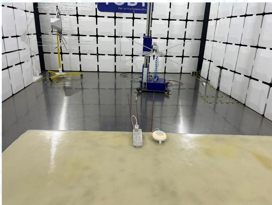
Photo of Setup for Radiated Emission (30MHz~1GHz)
