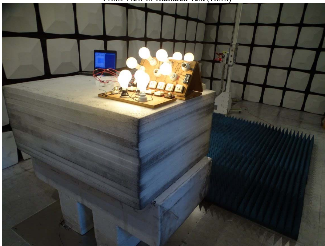
Front View of Radiated Test (Horn)
