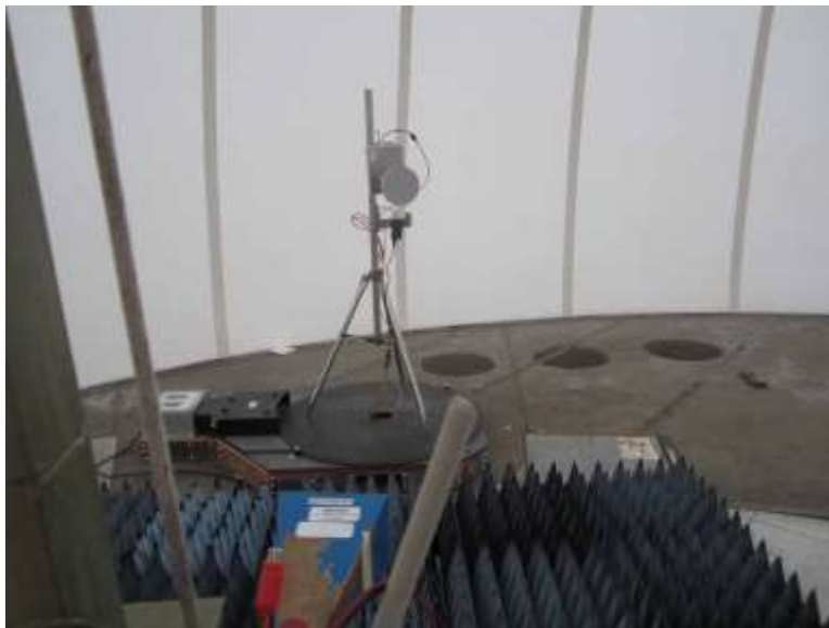
17.5dBi-26.5-40GHz, Cone placement
