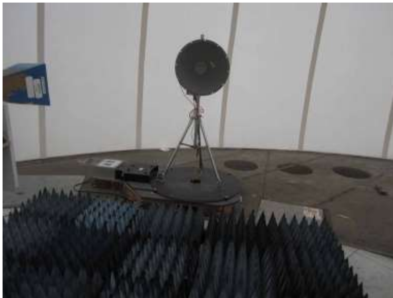
28dBi-26.5-40GHz, Cone placement
