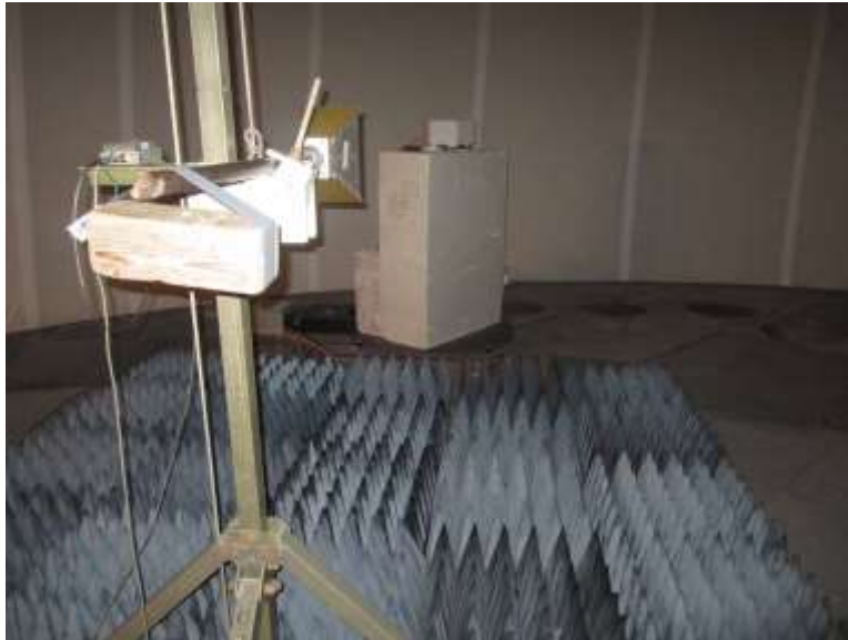
13dBi-Hex-1-12GHz, Cone placement
