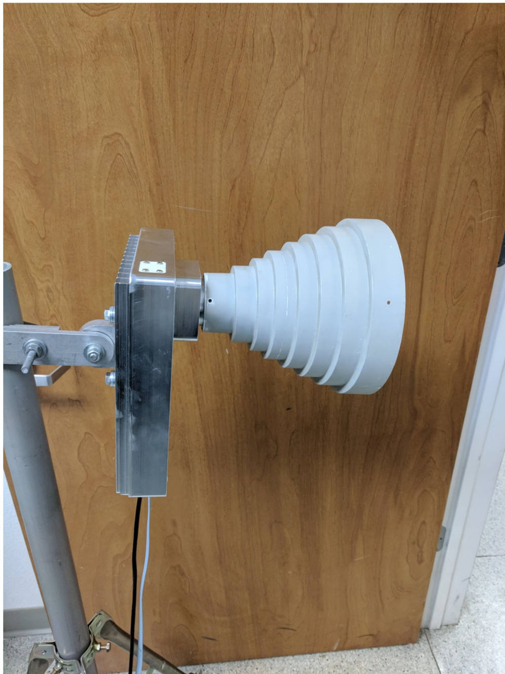
Single Horn 5 GHZ 30 degree Horn (17.5dBi) with external connectors as shown.
