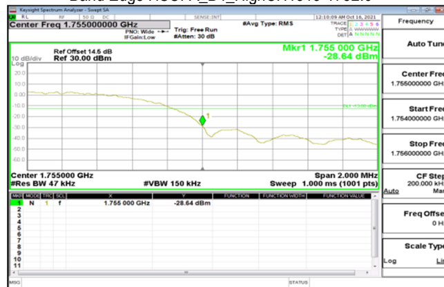
Band Edge HSUPA_B4_HighCH1513-1752.6
