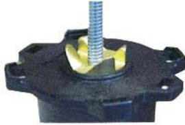
3. Carefully screw the MLOG Sensor into the threaded hole on the top of the clamp.
