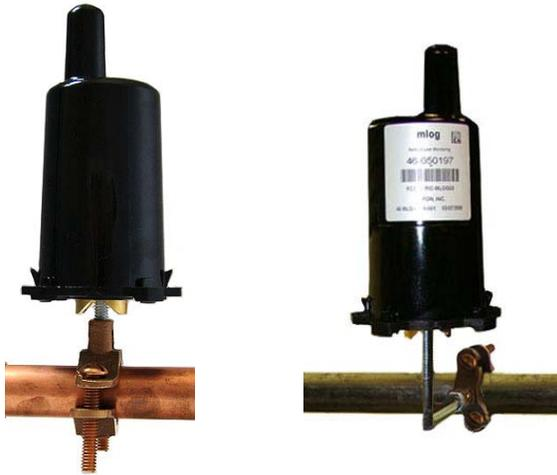
4. If the 90-degree angle mounting rod is used, place the pipe clamp as shown (back clamp plate over the screw from the top down for stability) and tighten the screw in an alternating fashion.
