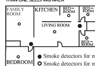
Figure 2: LOCATIONS FOR PLACING SMOKE DETECTORS FOR SINGLE-FLOOR RESIDENCE WITH MORE THAN ONE SLEEPING AREA
