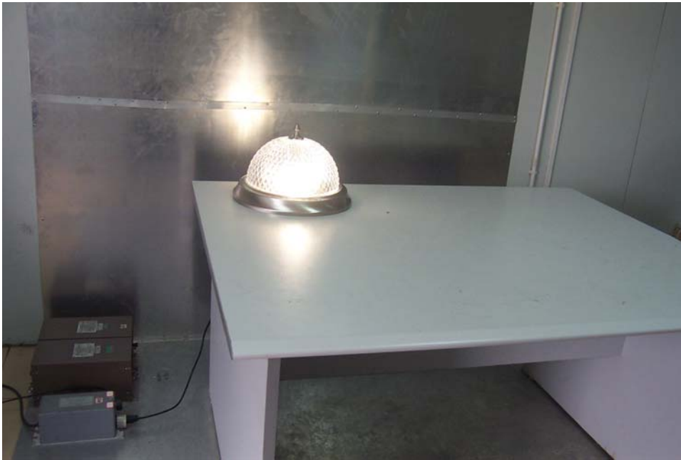
DW006: Conducted Emission– Side View
