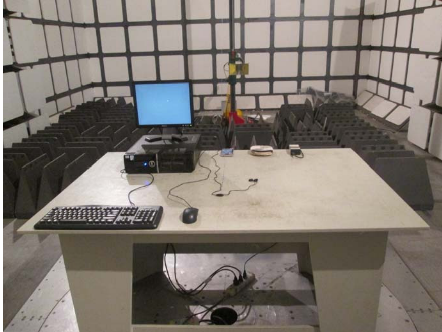
Radiated Emissions – Front View (Above 1 GHz)
