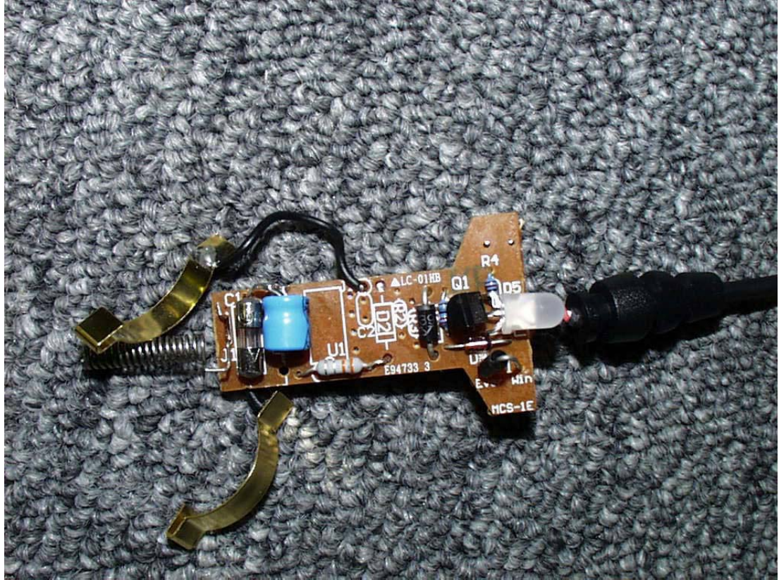
EUT: WIRELESS AUDIO FM TRANSMITTER. MODEL : 160732-00 Monster Stubby Cigarette Lighter connector PCB components side
