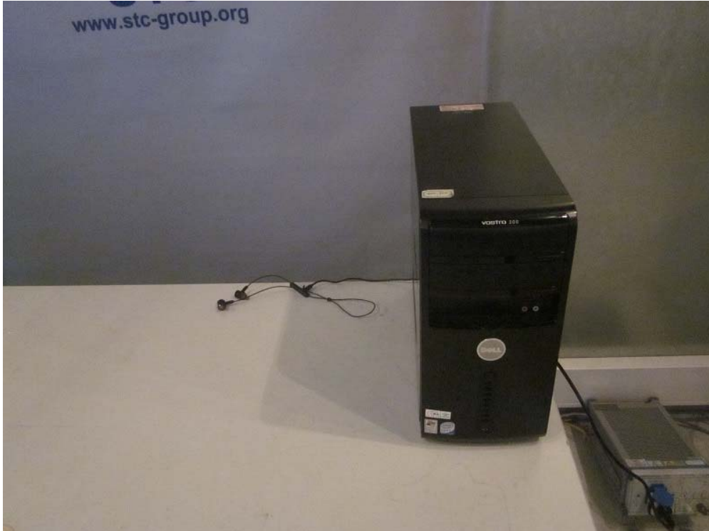
Measurement of Conducted Emission Test Set Up
