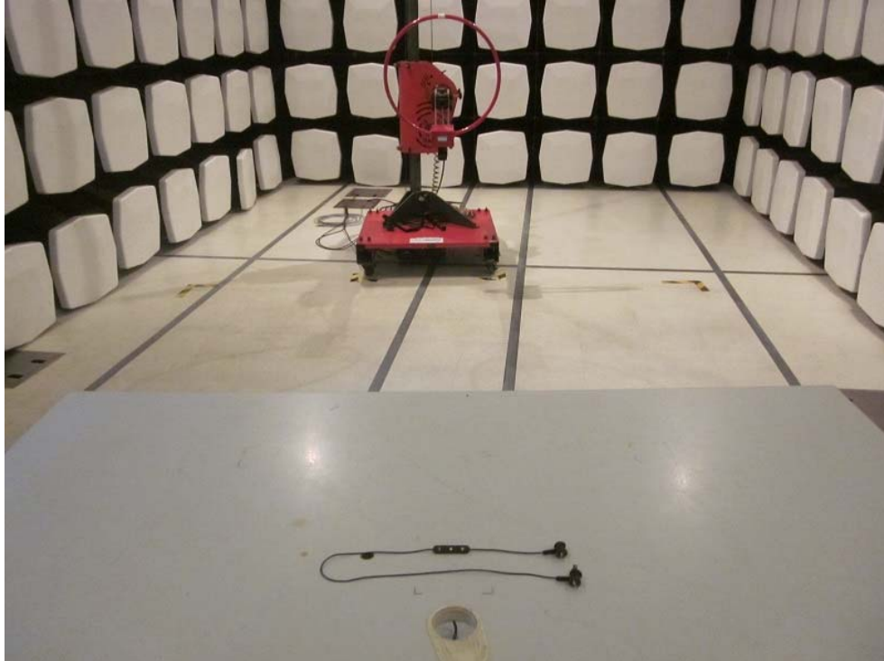
Measurement of Radiated Emission Test Set Up
