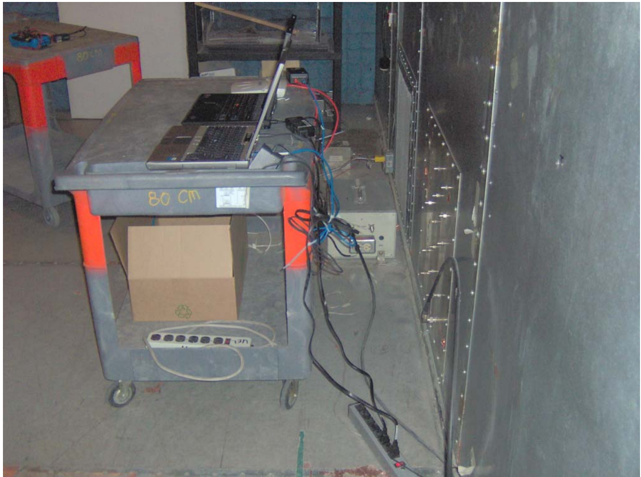
Test setup Configuration #2: The EUT is powered by the HUB (External Antenna Unit)
