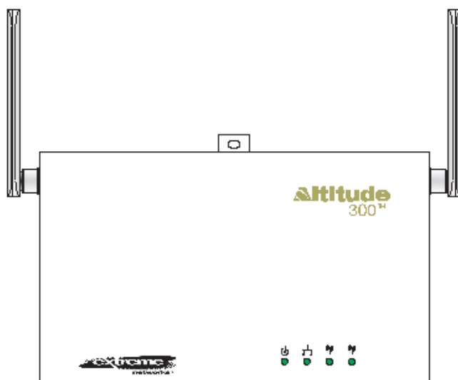
Figure 3: Altitude 300-2™ LED Indicators, Without Plastic Cover
