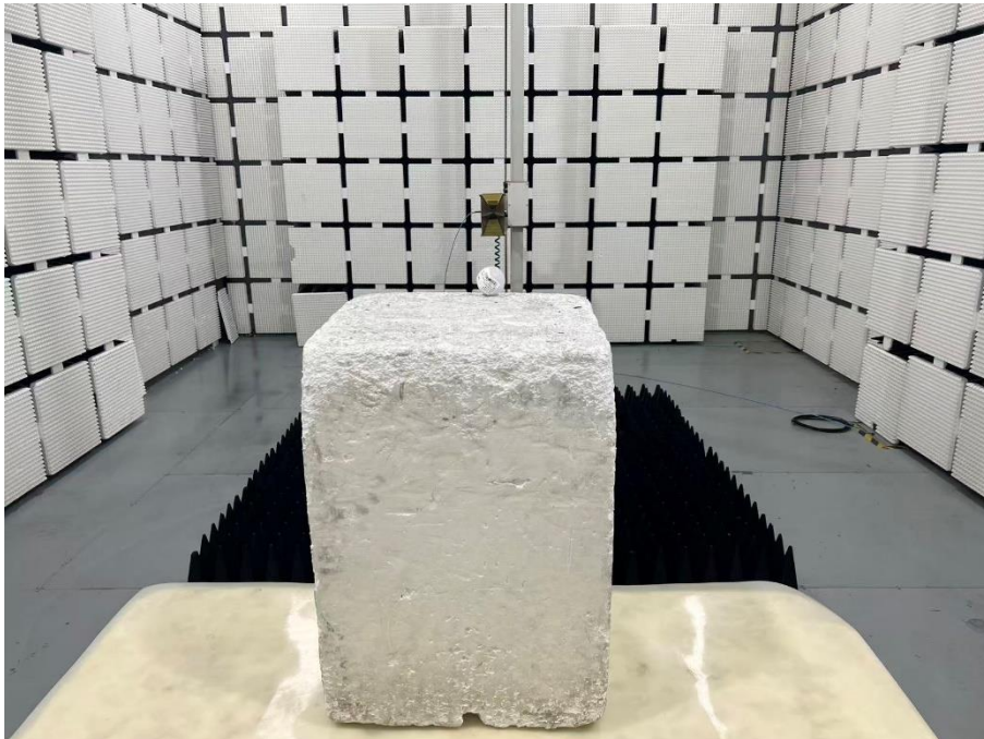
Set-up for Radiated Spurious Emission, Above 1GHz
