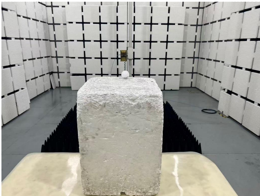
Set-up for Radiated Spurious Emission, Above 1GHz
