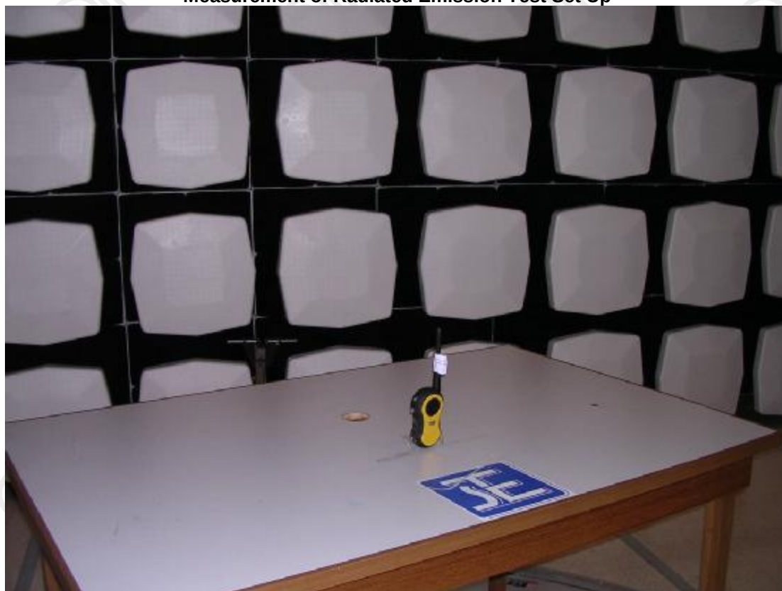
Measurement of Radiated Emission Test Set Up
