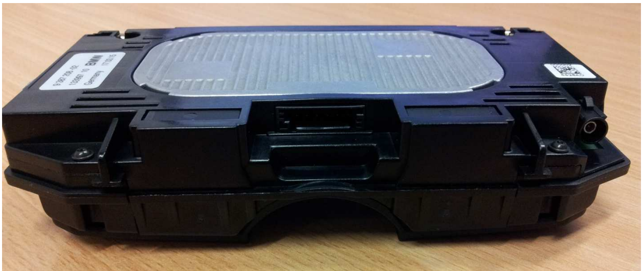
Side view with external antenna connector and system connector
