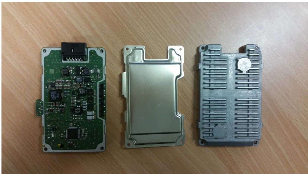
Main Board with Shielding and Cooling Element
