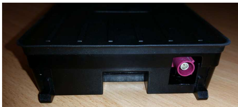
Side view with external antenna connector and system connector
