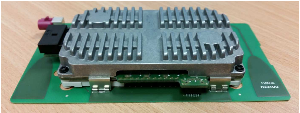
Antenna Board with Coil module, main board and cooling element (mounted)
