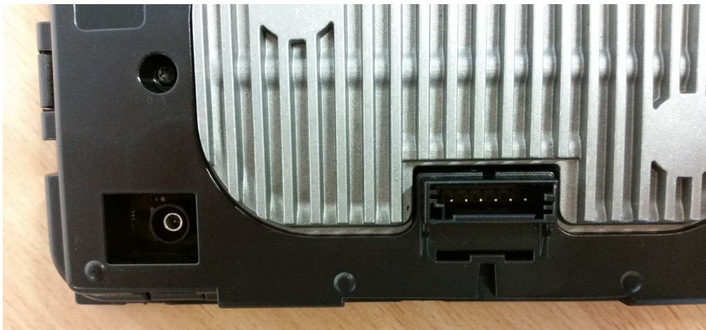
Bottom view (WCH-184a, WCH-184b)with System Connector and external antenna connector for Antenna coupler
