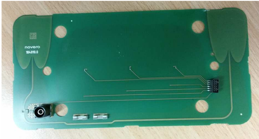
Top View Antenna Board with external antenna connector
