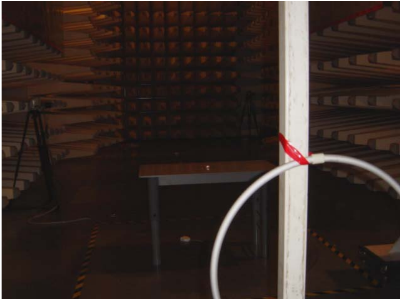
Set-up for Radiation Emission (Transceiver) – Loop Antenna
