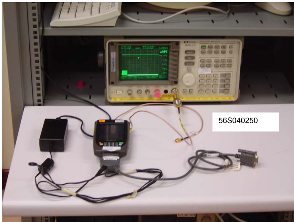
Spectrum Bandwidth Measurement Test Setup
