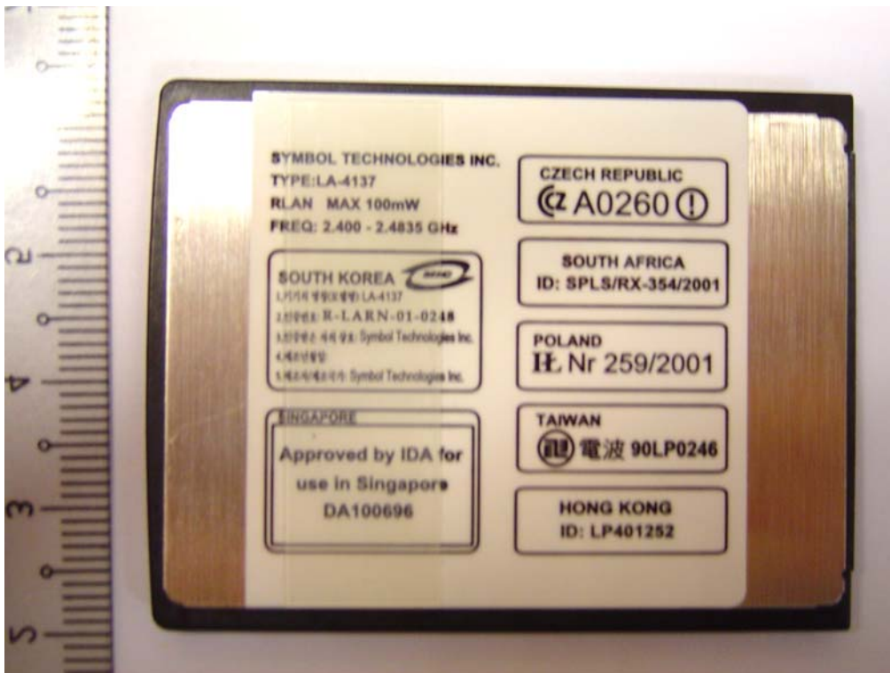
EUT RF Module – Bottom View
