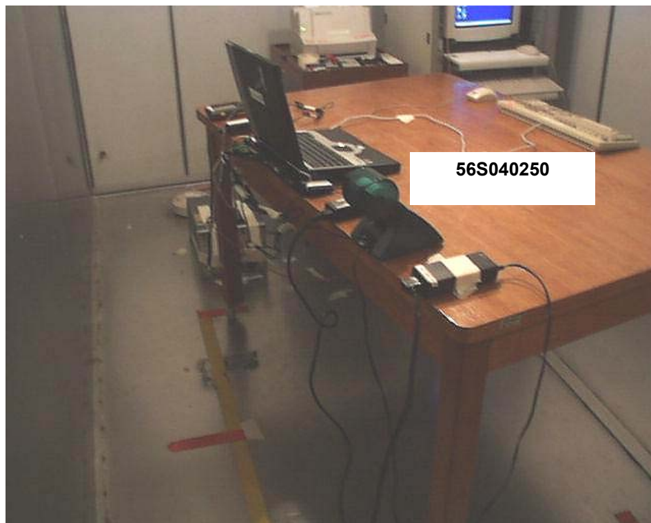
Conducted Emissions Setup (Rear View)
