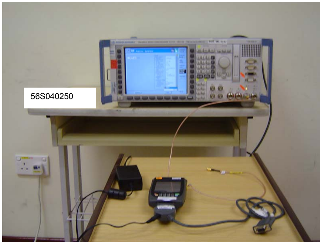
Maximum Peak Power Measurement Test Setup
