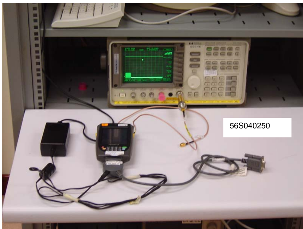
Number of Hopping Frequencies Measurement Test Setup
