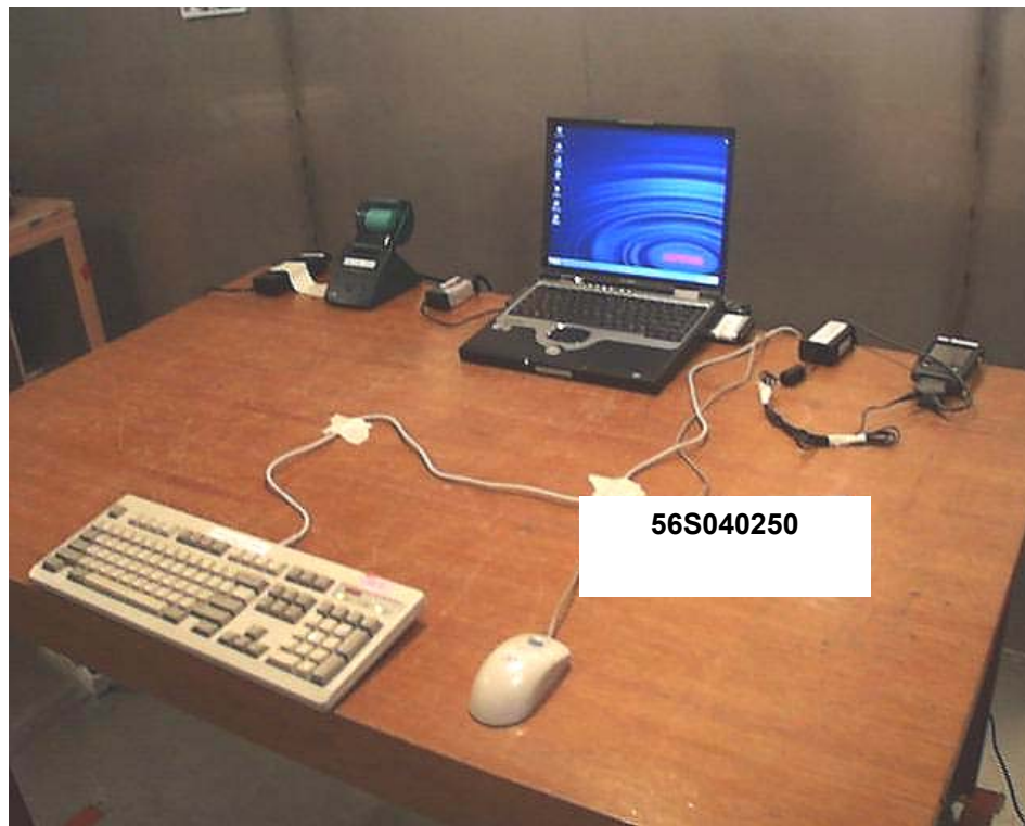
Conducted Emissions Setup (Front View)
