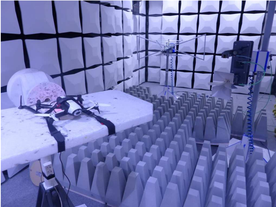
Photo 3: Test setup for radiated measurements (Enclosure, fully-anechoic chamber, 1-18 (15) GHz intentional radiator §15)
