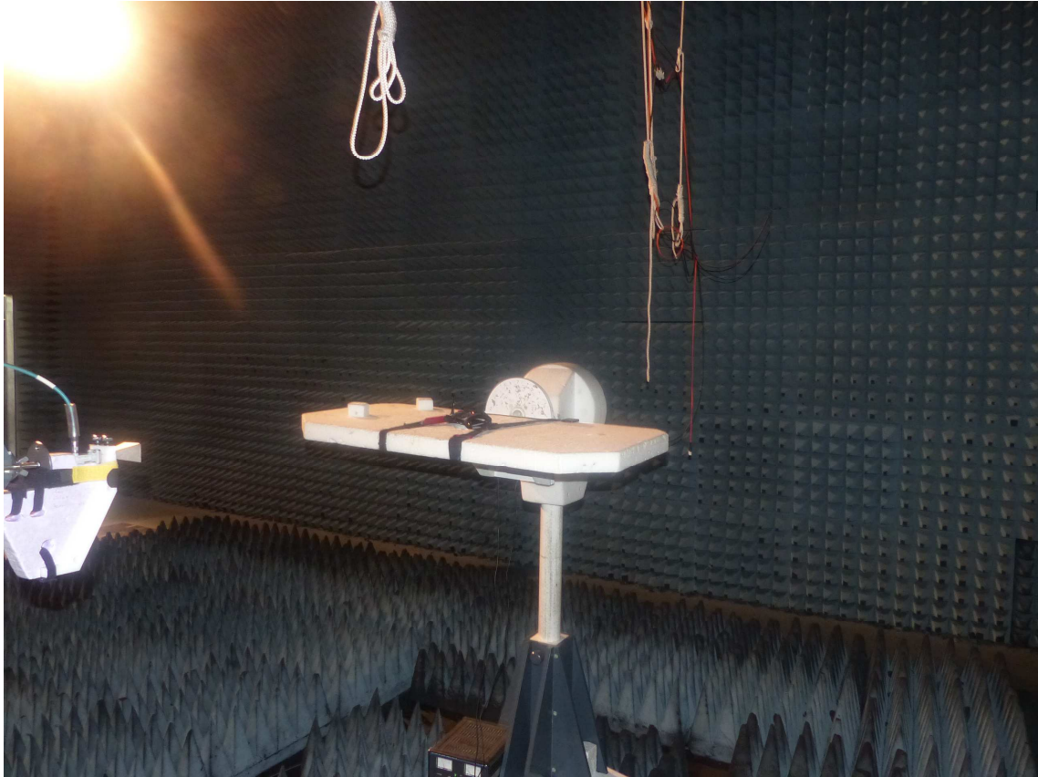
Photo 4: Test setup for radiated measurements (Enclosure, fully-anechoic chamber, 18-25 GHz, intentional radiator § 15.247)
