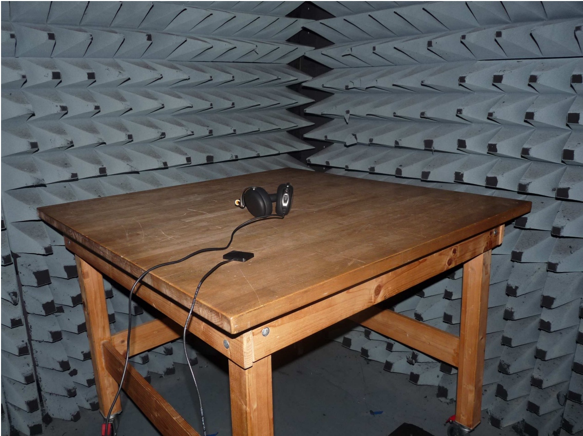
Photo 1: Test setup for radiated measurements (below 30 MHz)
