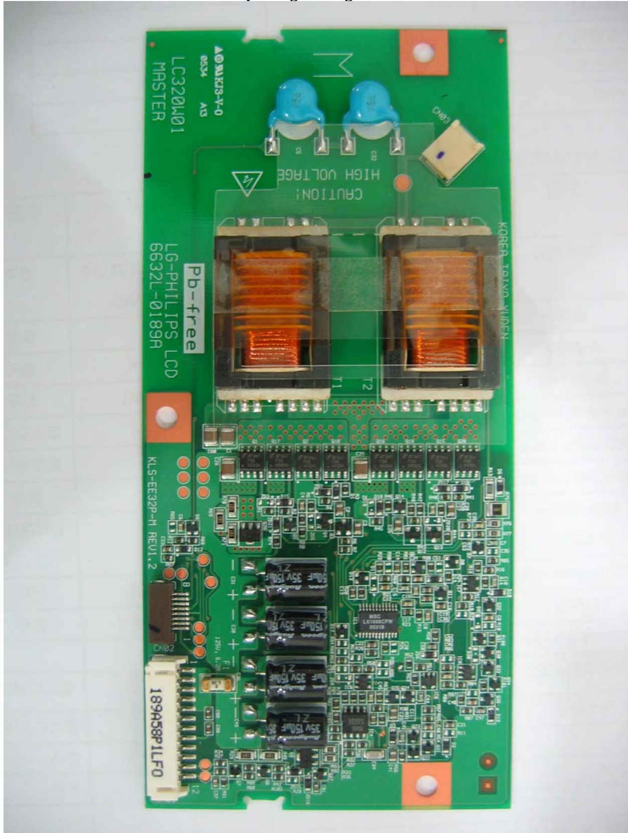
Top of high voltage board
